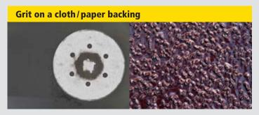
Grit on a cloth or paper backing is embedded in binder resin on the whole surface, and dust extraction is enabled by punched holes. The grit is glued together and has little space to incorporate dust, which can strongly influence the lifetime of the abrasive.
