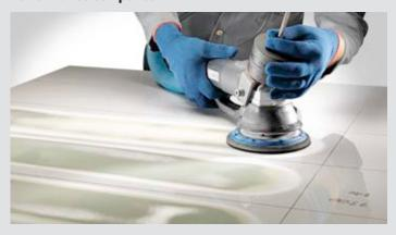
An oscillating sanding motion is used to sand a defined work area with a defined contact pressure. After a sanding time of three minutes, the work rate is compared by means of the material removal rate.
