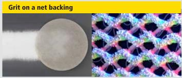
A net backing, consisting of a polyester fibre, is coated using a modern specific manufacturing procedure. Thanks to a sophisticated process, only the top fibre of the net is coated with grit. The inner, functional structure and the back of the abrasive with the siafast fastening loops remain free of grit.
