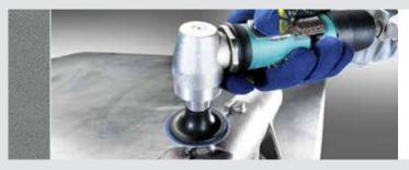
In addition to working on high-alloy and other hard to grind metals, 2707 siawat is also very suitable for stone, glass and plastic – covering different application steps including structuring.
