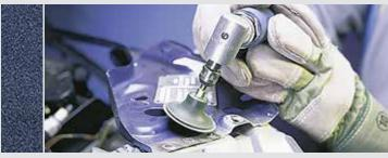
As a specialist product with high stock removal rates as well as excellent edge stability and tear resistance, 2820 siamet is suitable for a wide variety of jobs ranging from removal of rust or paint to preparation for welding – whether on unalloyed steels or non-ferrous metals.
